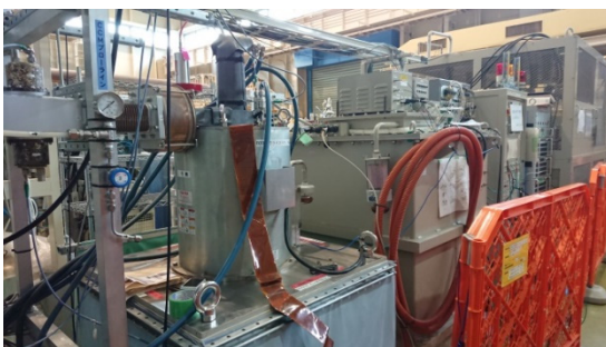
Figure 3: 10 MW Multi-Beam Klystron for CM1/2a (up), 800 kW Klystron for CCM (down).
