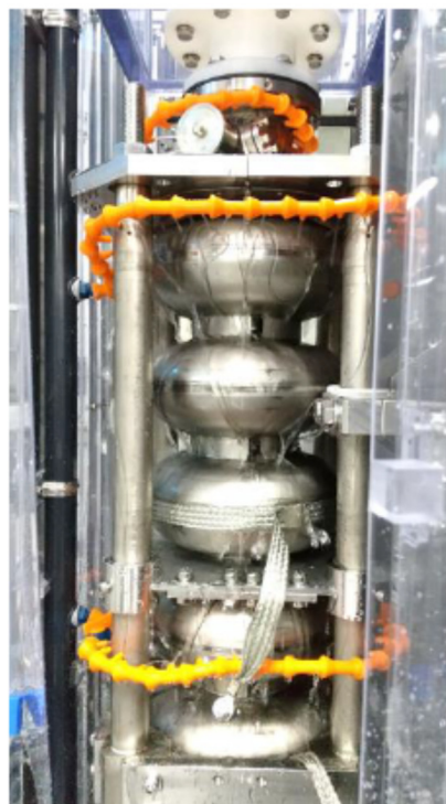
Figure 6: Cavity water cooling system using pure water.
