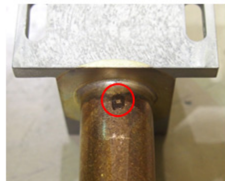
Figure 3: Cooling Water pipe pinhole.
