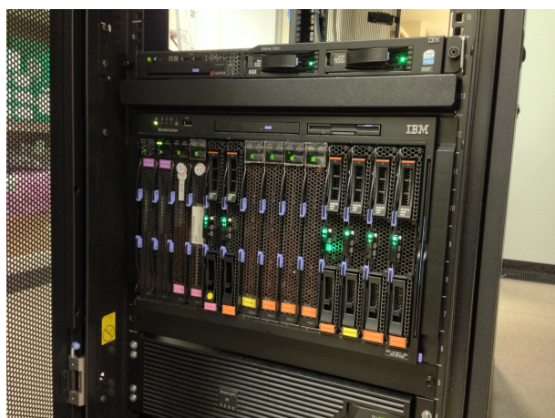
(a) An enclosure populated with 14 blades.
