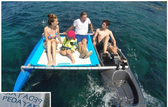
In the spirit of the Polynesian pendulum pirogues that crossed the Pacific, a stabilising side float is mounted on one side of the **PEDAYAK** and held together with a structure and a large trampoline, the same as that of the **PEDAYAK DUO**. But unlike the **DUO**, there is only one person pedaling.
