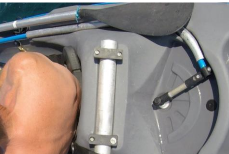
Steering control stick and tiller: right or left direction
