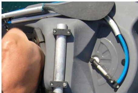
Steering control stick and tiller: right or left direction
