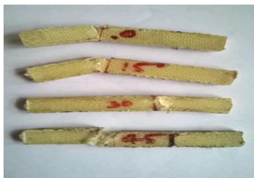
Fig 7: Impact test specimens with filler material after testing
