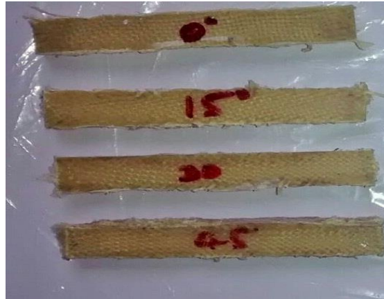
Fig 4: Impact test specimens without filler material before testing
