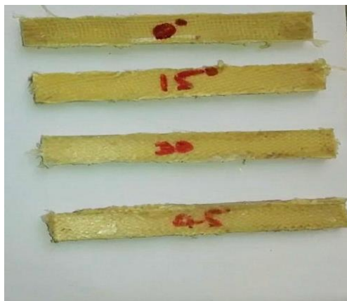
Fig 3: Impact test specimens with filler material before testing
