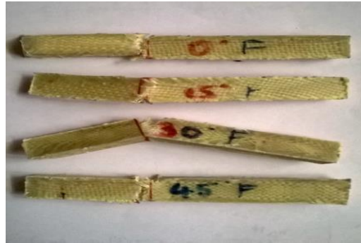
Fig 8: Impact test specimens without filler material after testing
