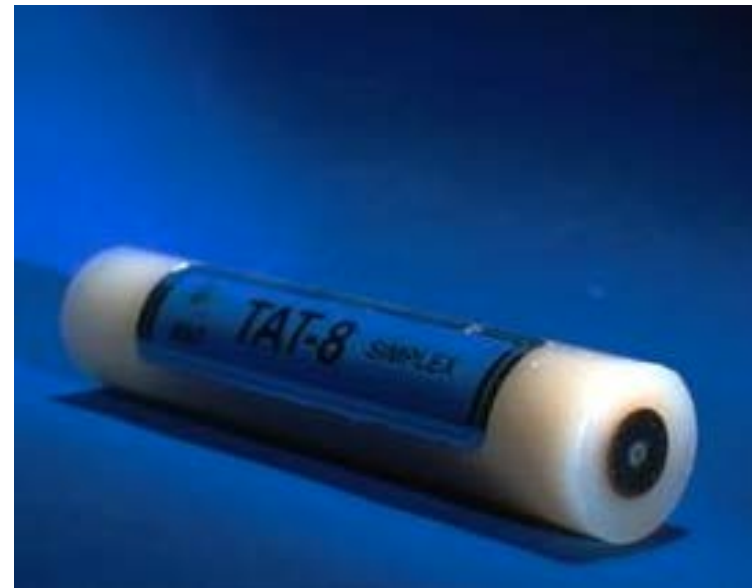
First fiber optic submarine cable - TAT-8 (1988)
