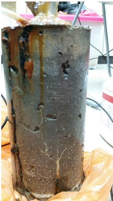
Fig. 11. Rust stain emerged from concrete cracks.
