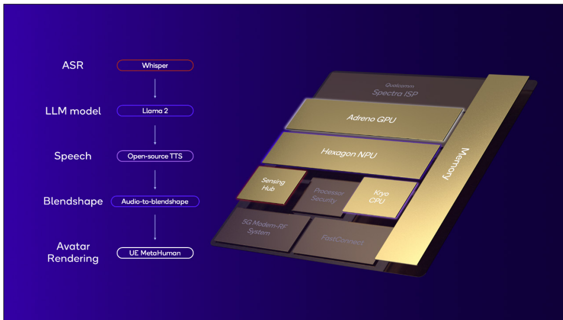
Figure 8: The personal assistant with an avatar utilizes all the diverse processors of the Qualcomm AI Engine.
