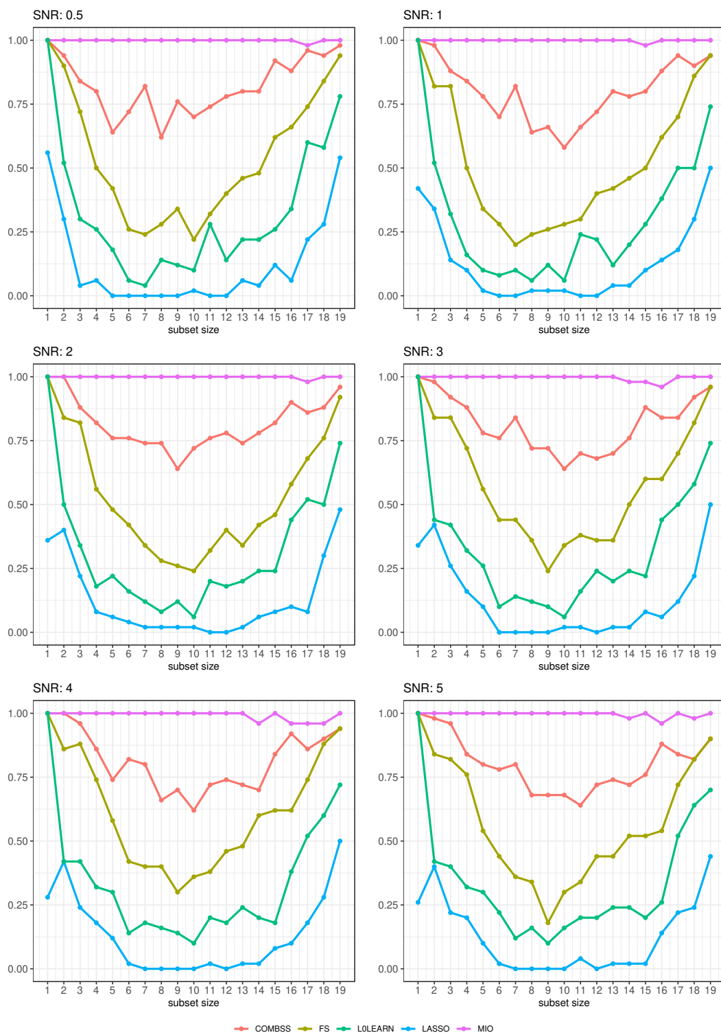
Fig. 6: Frequency (over 50 replications) of retrieving the exact best subset for any subset size from k = 1, \dots, p for beta-type 3 case.
