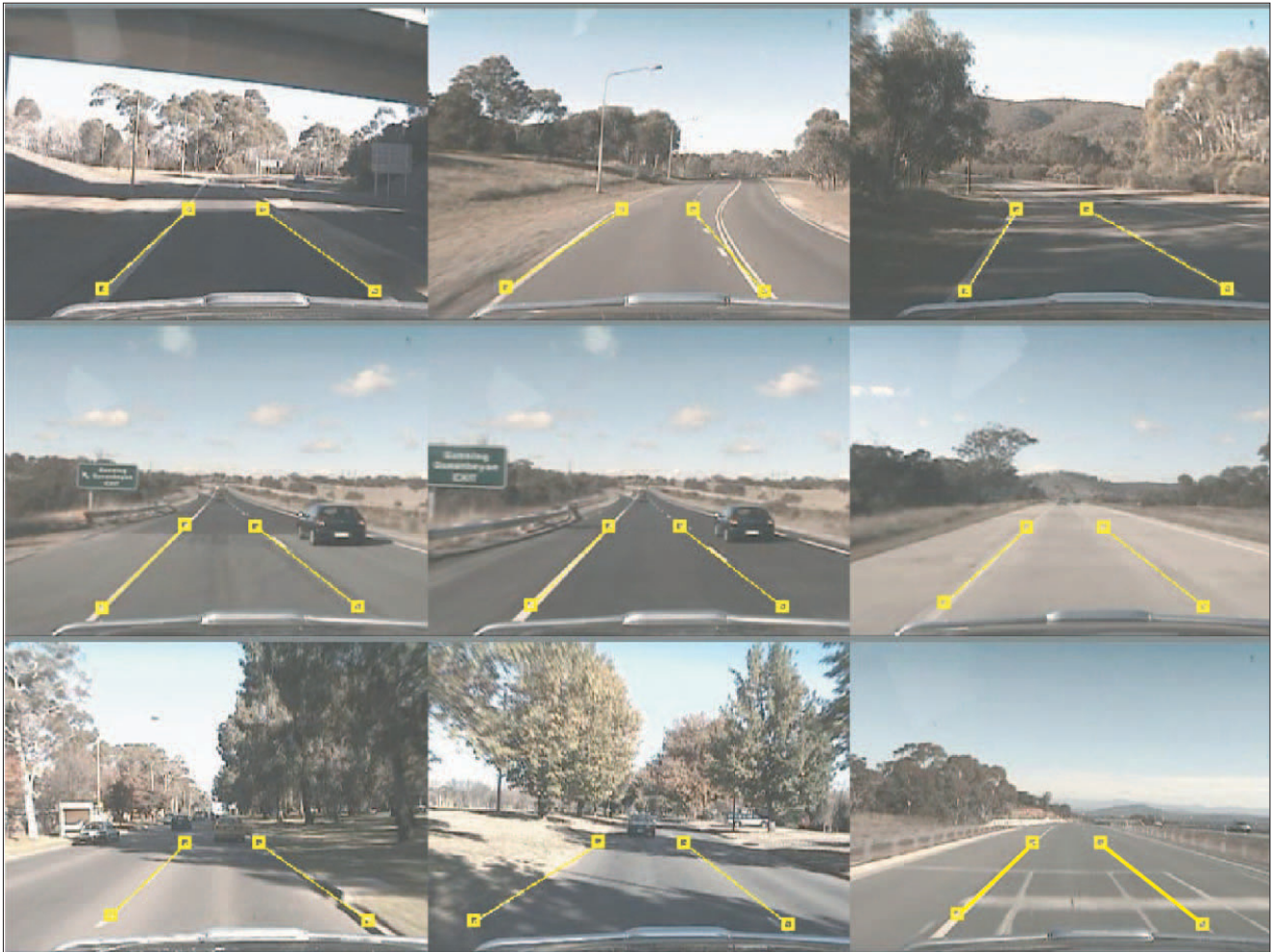
Figure 3. Lane tracker results. Yellow lines indicate the estimated lane boundary. Tracking is robust against shadows, obstacles, and misleading lines on the road.
