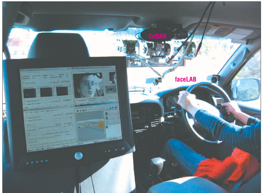
Figure 1. The Transport Research Experimental Vehicle uses two vision platforms: the CeDAR (Cable Drive Active Vision Robot) active-vision head and faceLAB passive stereo cameras.
