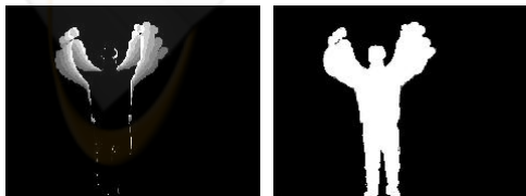
Figure 1: Illustration of the MHI (left) and MEI (right) in a case where a person is raising both hands.
