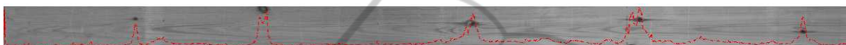
Figure 6: A cropped section of a board with 1-D projection signal plotted over.
