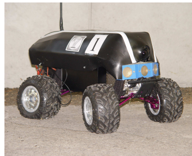
Figure 2: The Teleoperated OutdoorMERLIN Robot.
