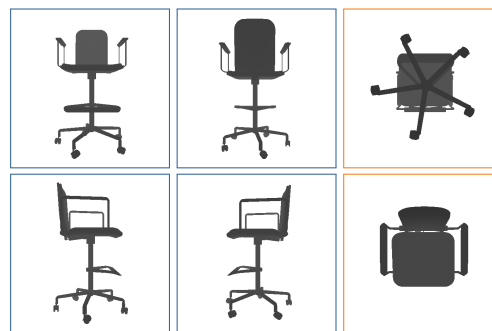
Figure 1: Example of the six depth maps used for the analysis of a chair 3D model. Notice how there are four similar side views ( blue boxes ) and the top and bottom ones ( orange boxes ).
