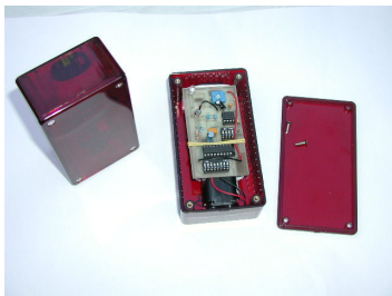
Fig. 5. Infrared location beacons.
