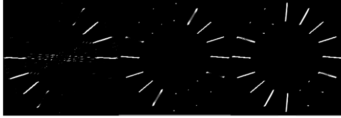
Figure 2. Reconstructed images for \nu = 66^\circ . From left to right: FBP, TV, DTV.
