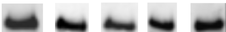
Figure 3. Pure protein bands (NESP) showing bimodal leakage and smears on top of the band. All spots were taken from "Desharnais, P., J.F. Naud, and C. Ayotte, Desialylation improves the detection of recombinant erythropoietins in urine samples analyzed by SDS-PAGE . Drug Test Anal , 2013. 5 (11-12): p. 870-6". [5]
