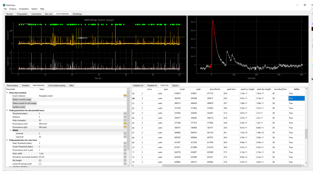
Figure 2: PatchView mini-event analysis GUI. Top left: large-scale view of the trace. The top yellow line is the original trace. The bottom white trace is a deconvolved trace with separate threshold (red horizontal line). Top right: currently selected event. Bottom left: parameters panel. Bottom right: table for detected events' detailed quantification.
