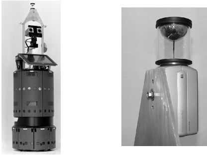
Figure 2: (Left) Experimental platform PERSES, an extended version of a B21 robot, equipped with an omnidirectional imaging system on top. (Right) The omnidirectional vision system consists of a vertically oriented color camera (digital Sony CCD camera DFW-VL 500 with IEEE 1394 connection) and a middle-size spherical mirror (from Accowle).
