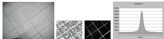
Figure 4: General idea of our vision-based odometry correction considering the regular structure of the market floor: (from left to right) a) image of the floor in front of the robot, b) local orientation or structure tensors [5] (orientations coded as gray values), c) confidences of local orientations (low-black, high-white), d) histogram of confidence-weighted local orientations (interval 0^\circ - 90^\circ ). The dominant orientation (center of gravity) is a significant measure for the accurate orientation of the robot with respect to the global orientation of the tiles.
