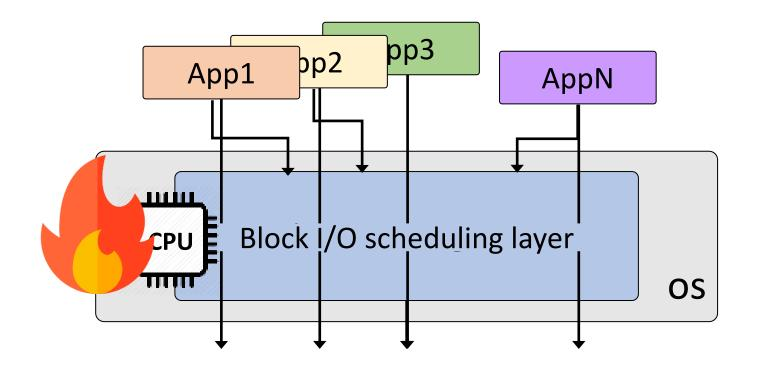
Saving host CPU cycles by offloading I/O scheduling function to device
