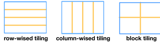
Figure 1: Three tiling methods for 2-dimensional arrays.
