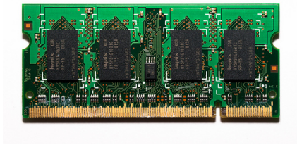
Figure 2: A SO-DIMM with its memory chips.
