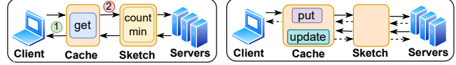
Figure 3: In-switch key-value store cache implemented using SwitchVM. ① and ② show the flow of cache hit and miss respectively. Cache-get/put/update and count-min represent DPFs and the pipeline they are executed on.
