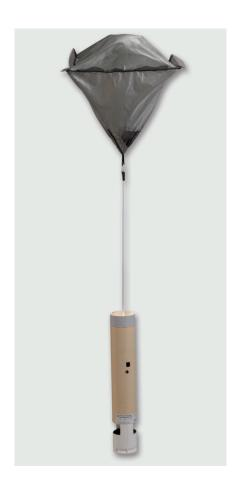
tropical cyclone reconnaissance and research, data acquisition over oceans as input for Numerical Weather Prediction (NWP) models, as well as in various field campaigns to acquire data for meteorological research and for validation of other airborne instrumentation. It has been used from low, 1500 ft, to high, 66 kft, altitude drops. The RD94 transmits data using a narrow bandwidth FSK (Frequency Shift Key) modulation in the 403 MHz
