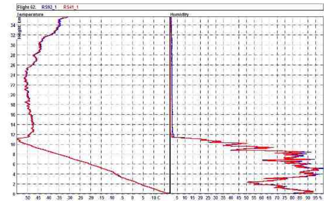
Figure 4.2. Example temperature and humidity profile of a high latitude daytime sounding. Tropopause is at about 11 km height and temperature drops down to -55°C.
