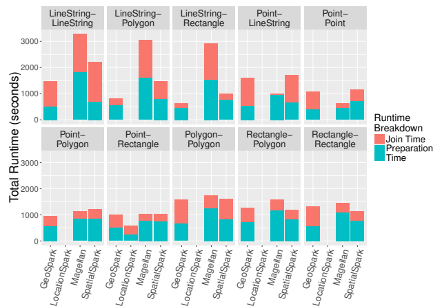
Figure 16: Total runtime cost breakdown for spatial joins between various geometric objects on a single node
