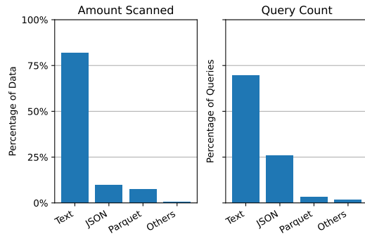
Figure 12: Storage Format on S3: The format of external table data, either read by COPY or within an external table scan.
