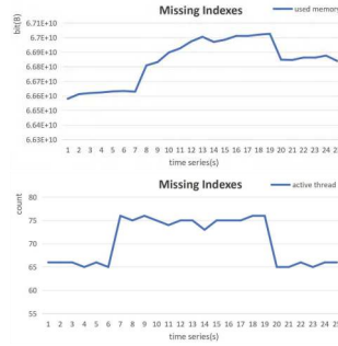
Figure 4: Used Memory and Active Thread of DBPA under missing indexes anomaly.
