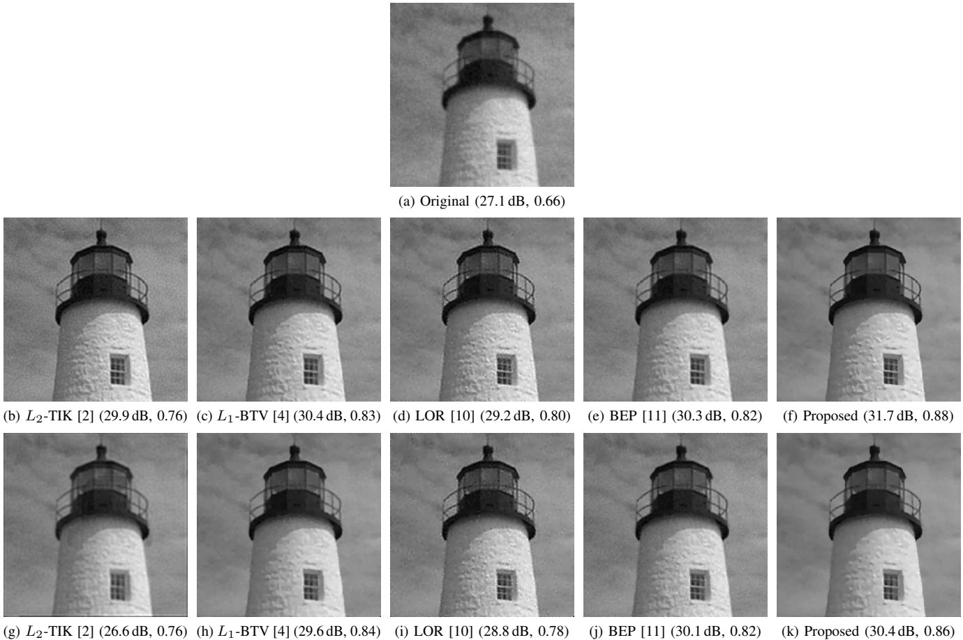
Fig. 4: Super-resolution on the Lighthouse dataset with PSNR and SSIM measures in brackets ( K = 8 frames, magnification s = 2 ). Top row: original, low-resolution frame. Middle row: super-resolution using exact subpixel motion. Bottom row: super-resolution under inaccurate subpixel motion.
