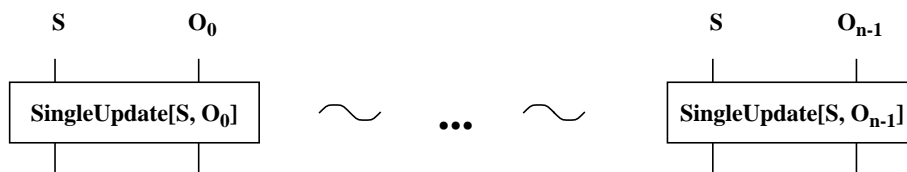
Figure 14 : Updating the State Information of all Registered Observers O_0, \dots, O_{n-1} with Subject S
