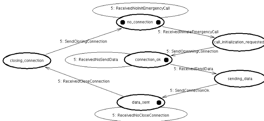
Fig. 3. State Transition Diagram of the Mobile Phone Logic Component
