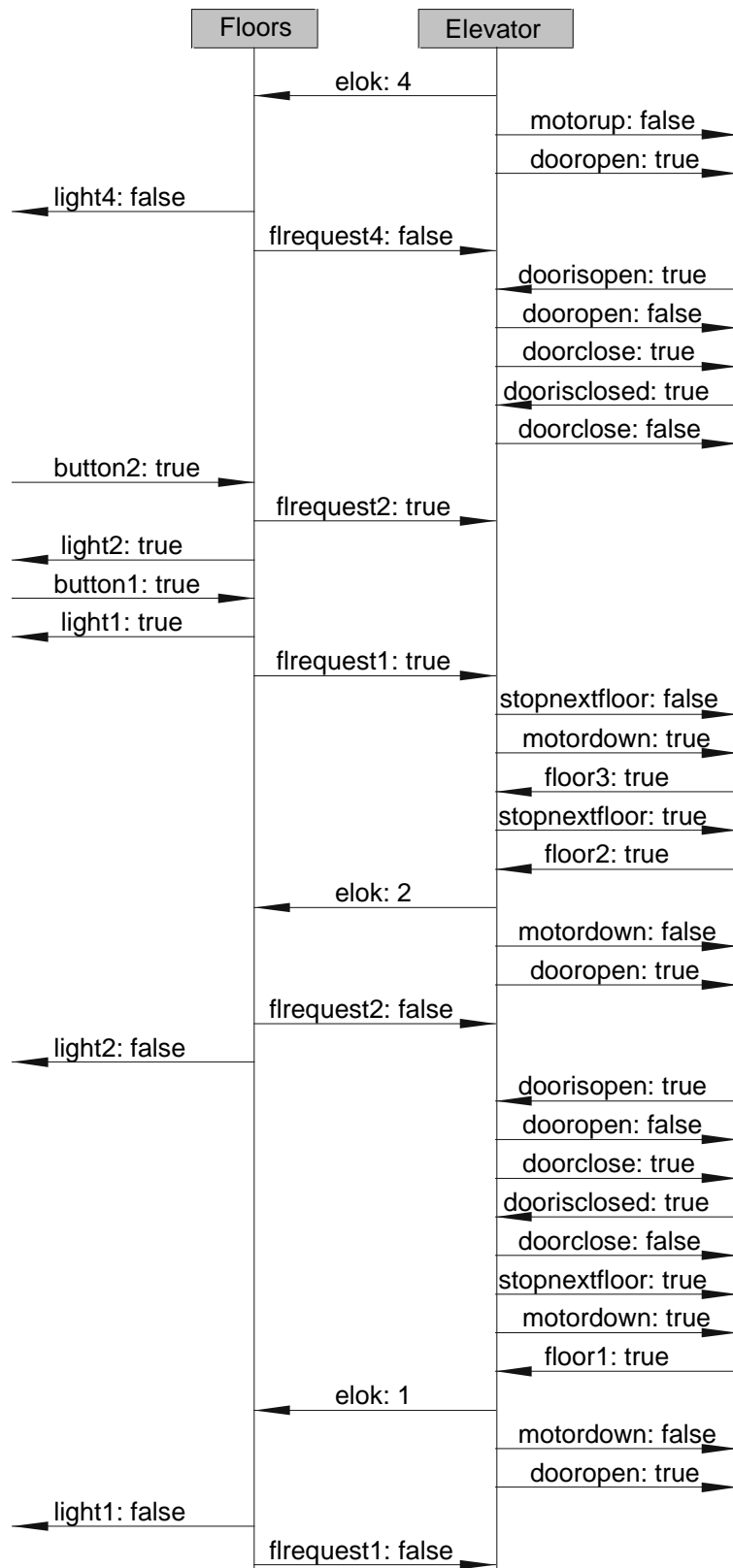
Figure A-6: EET Elevator Control System (continuation)
